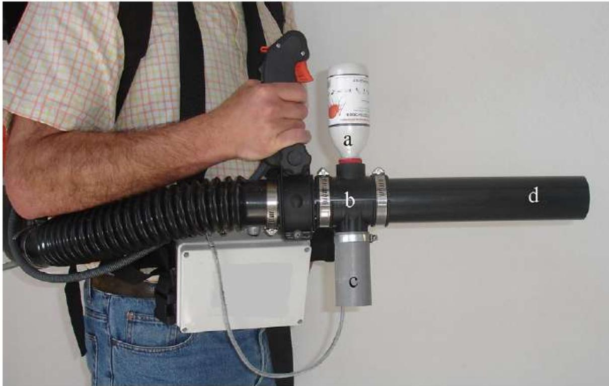
**Fig. 1 – Mechanical blower: a) bottle containing beneficial organisms; b) extraction system; c) electromagnet; d) air diffuser.**
