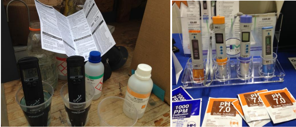
Figure 1: Regular use of meters to measure EC levels. Photos by L. Pundt
