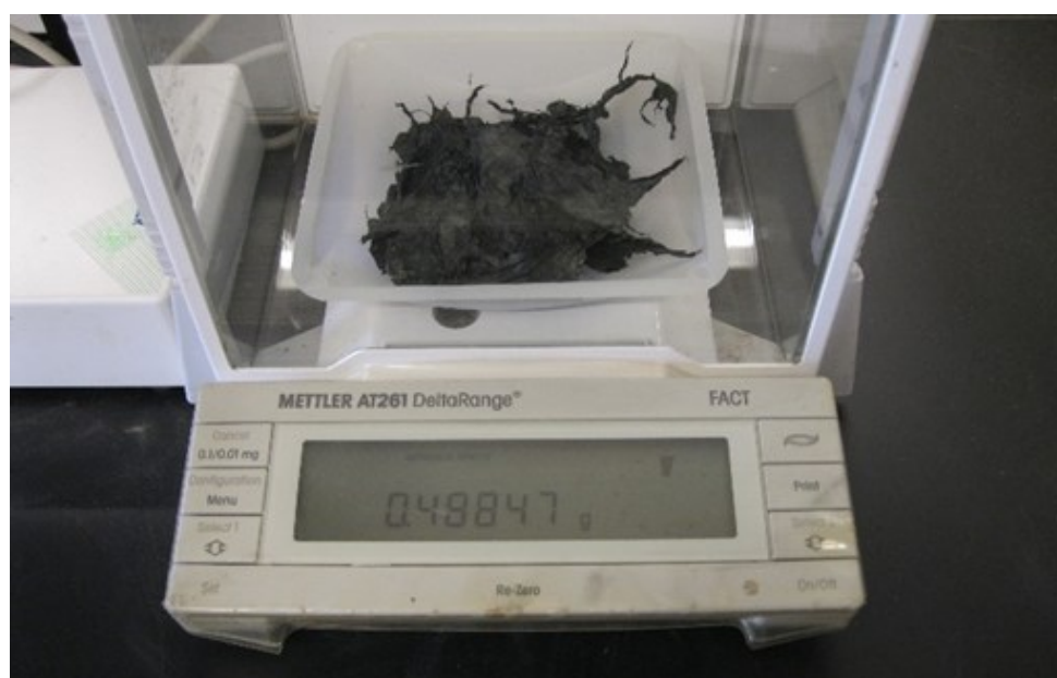
Figure 4. Weighing of plastic mulch fragments in a precision balance.
