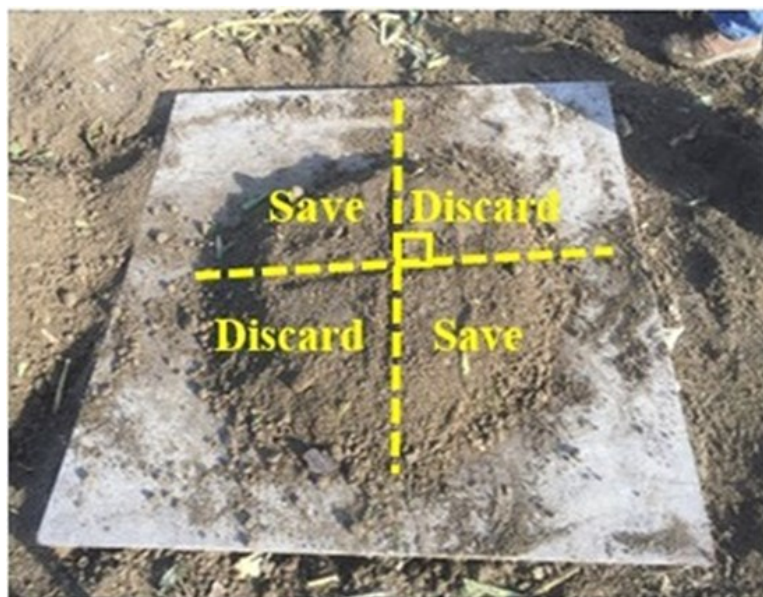
Figure 1. Quartering method of soil sampling.
