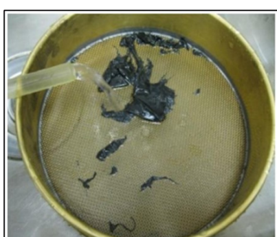
Figure 3. Process of recovering mulch fragments from soil sample.
